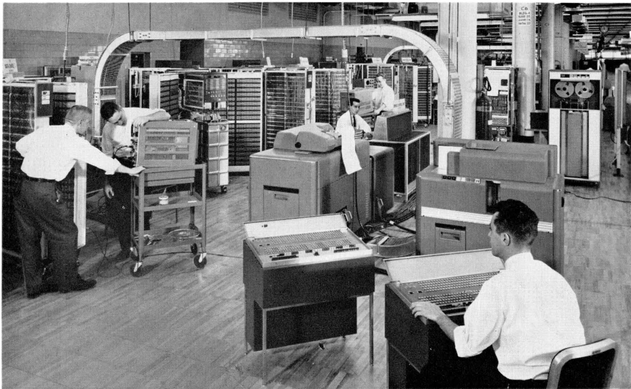
Figure 2. In-manufacture Test of Large-scale IBM Data Processing System
